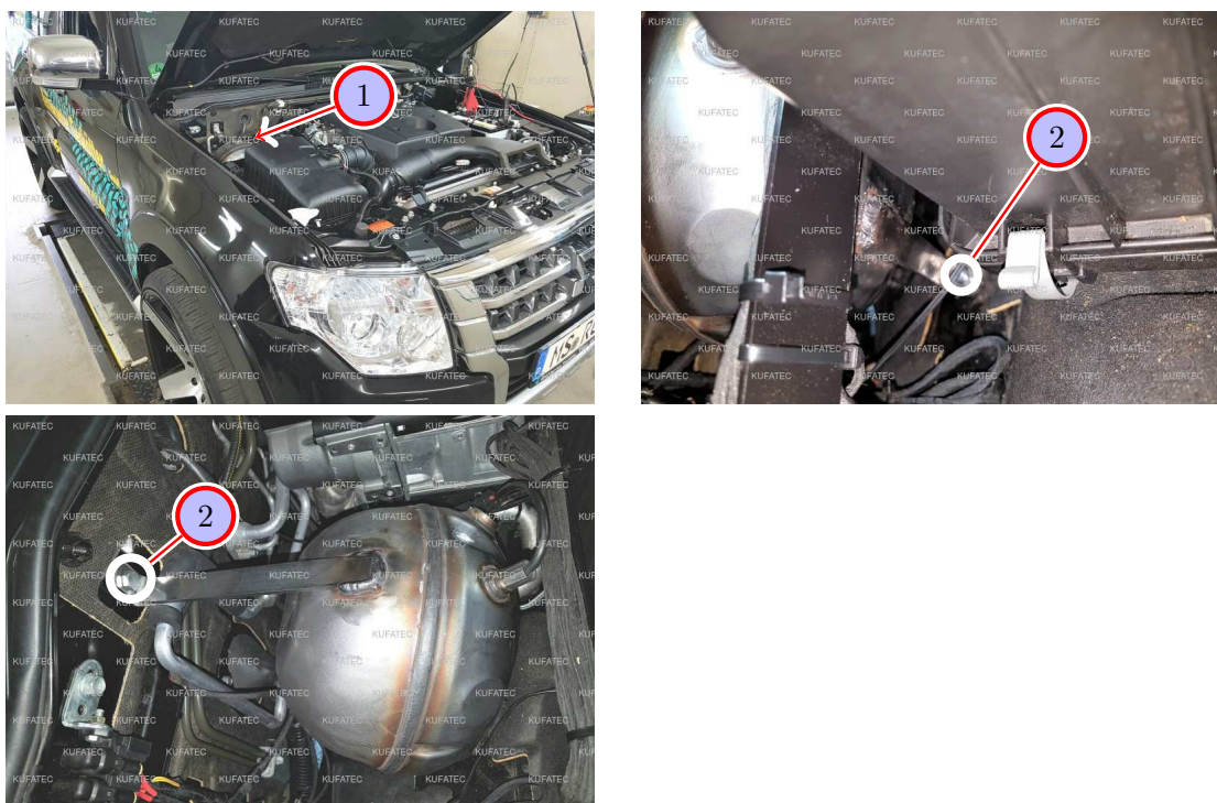
Figure 12: Installation front sound generator
