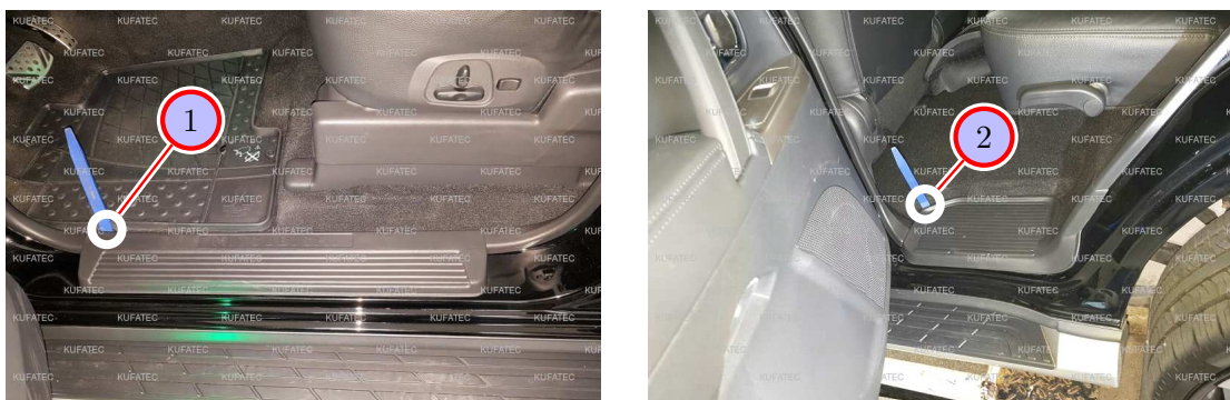
Figure 5: Removing trim panels driver's side
